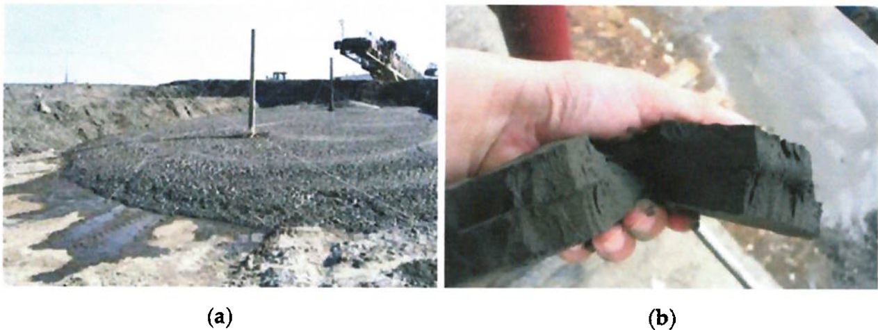
Figure 20. Consistency of (a) centrifuged wet tailings filter cake, and (b) filtered dry tailings filter cake.
