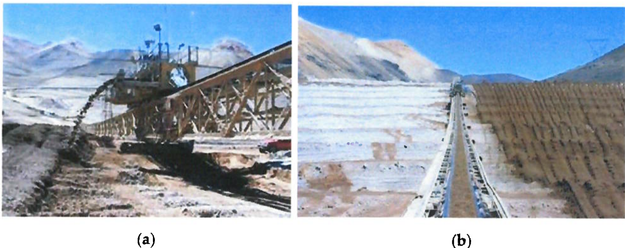
Figure 21. Dry stacking of filtered tailings at La Coipa, Atacama region, northern Chile, showing (a) stacker, and (b) overall stack [29].
